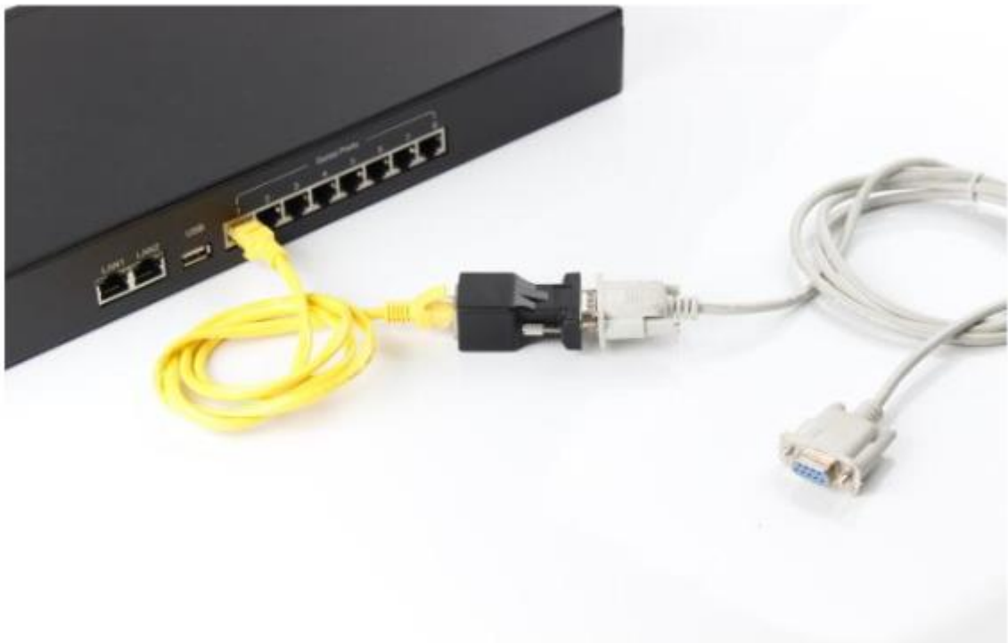
Figure 2. serial port connection between N668 and PC
