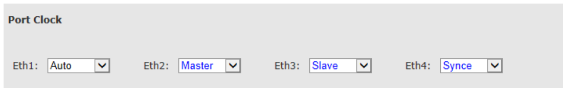
Figure 10-6 Advanced Config Page: Synchronization – SyncE Port Clock
