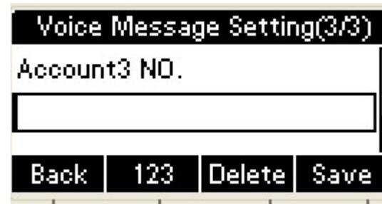
8. Press the OK key on the phone keyboard or the Save soft key to save and return to message interface.
