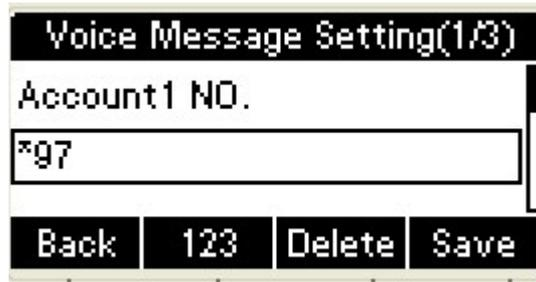
6. Press the Down key on the phone keyboard to set account 2, input the Visit account number of voice message( For example: \*99), press 123 soft key to switch the input methods :
