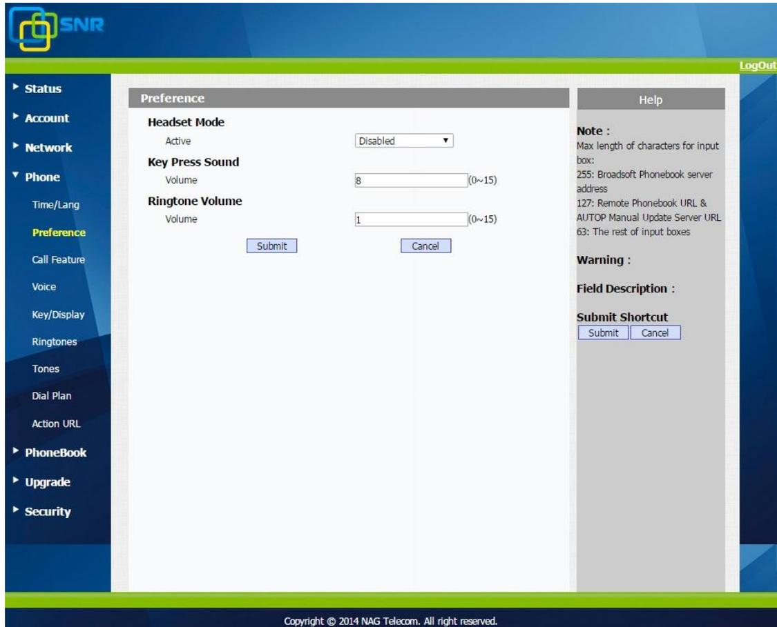
The screenshot shows the SNR web interface for configuring phone preferences. The left sidebar lists various settings categories, with 'Preference' highlighted. The main area is divided into three sections: 'Headset Mode' (Active: Disabled), 'Key Press Sound' (Volume: 8), and 'Ringtone Volume' (Volume: 1). Each section has a 'Submit' and 'Cancel' button. A 'Help' sidebar on the right provides additional information, including a note on input box lengths, a warning, and a submit shortcut.
