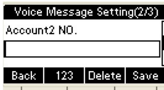
7. Press the Down key on the phone keyboard to set account 3, input voice message visit account number( For example: \*100), press 123 soft key to switch the input methods
