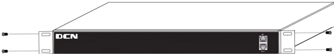
Figure 3-1 S7550 series switch install sketch map on the rack using stock
