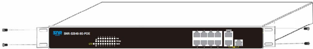
Fig 2-1 Fasten the Brackets to the Switch
