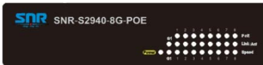
Fig 1-6 SNR-S2940-8G-POE LED diagram
