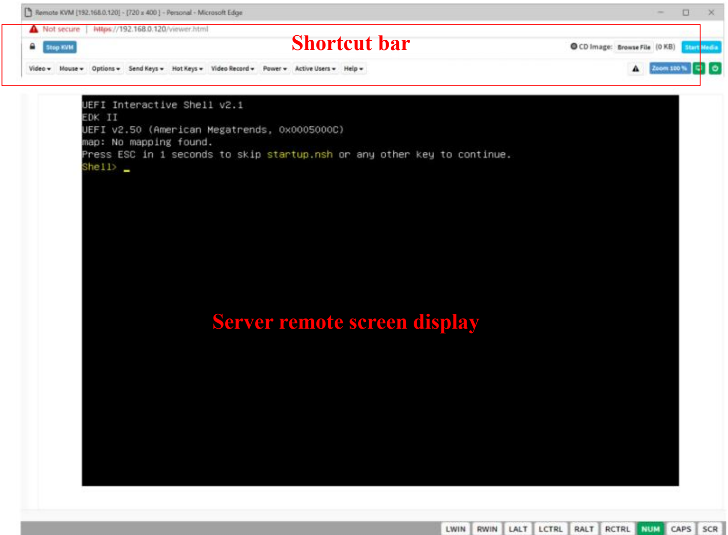
Figure 7-13 Composition of KVM interface
