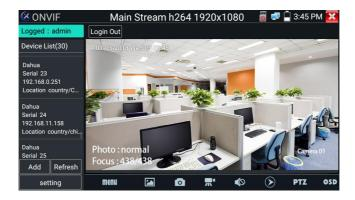
Click the button "Refresh", tester will scan the ONVIF camera again. Click the newly displayed ONVIF camera on the "Device List". The tester will show the IP camera's relative information and settings.
