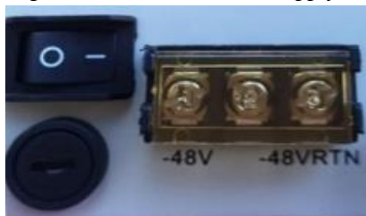
Figure 3-4 -48VDC Power Supply PIN Definition
