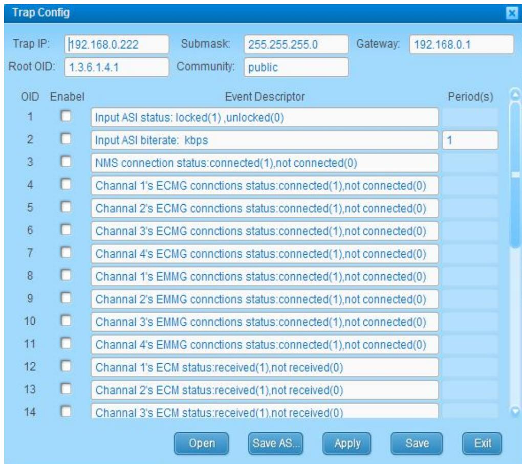
Trap IP: set the IP address of Trap host.
