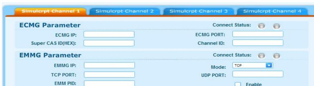
**ECMG Connect Status:** the green light turns on when the ECMG works correctly.
