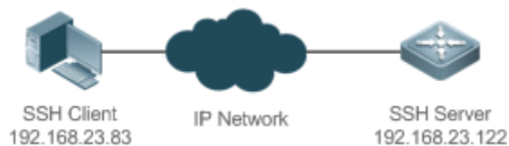
Figure 10-30 Networking Topology of SSH File Transfer
