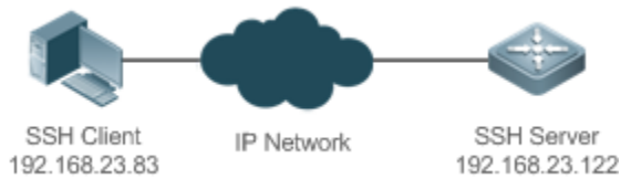
Figure 10-26 Networking Topology of SSH Device Management
