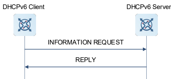
Figure 1-1 Message Exchange Using the Stateless Service
