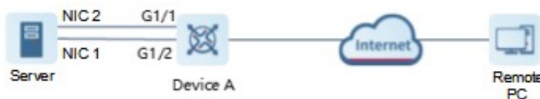
Figure 1-1 Topology for Configuring Automatic Server Deployment over a Preferred LACP AP
