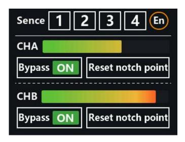
This interface mainly includes scene switching, signal level display, channel bypass, reset notch point, screen lock, language switching.
