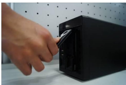
③ Pull the HDD knob up when you put the HDD into the box in case the knob buckle may strike the front panel.
