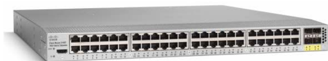
Figure 2. Cisco Nexus 2148T Fabric Extender Provides 48 Gigabit Ethernet Server Ports in a Compact 1RU Chassis
