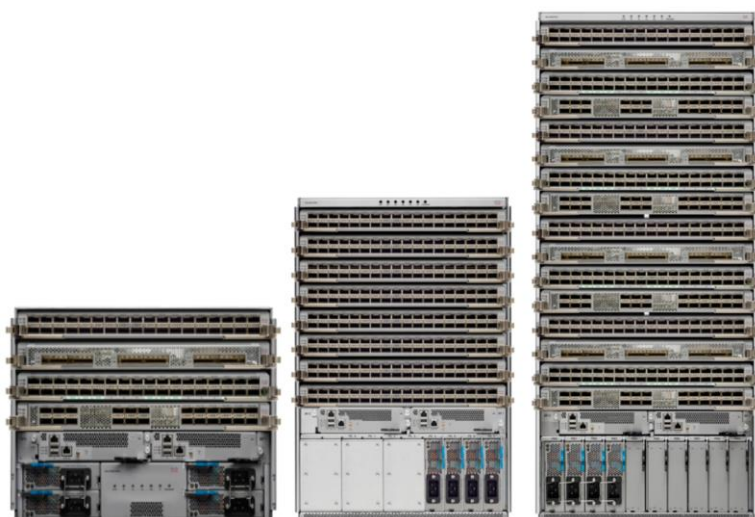
Figure 1. Cisco NCS 5504, Cisco NCS 5508 and NCS 5516 chassis
