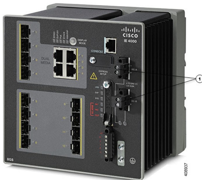
Figure 10 Removing the Power Connectors from the Switch
