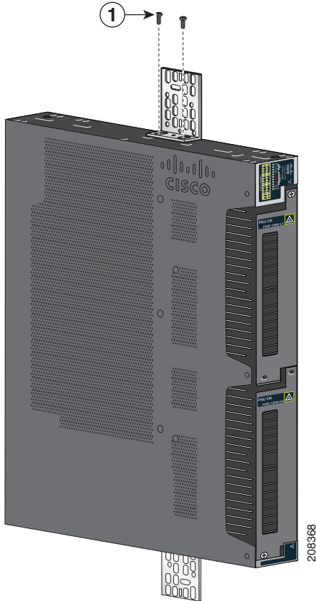
Figure 20 Attaching 19-inch Rack Brackets
