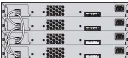
Figure 7. Four Member Stack with 0.5-Meter Cables
