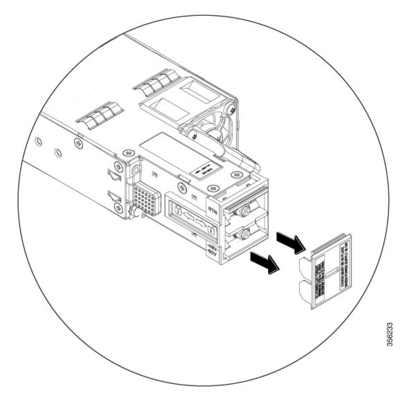
**b.** Loosen and unscrew the two nuts on the terminal box. The terminal box has two slots for power terminals. Each terminal has a nut that you use to fasten the power cable to the terminal.
