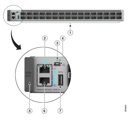
Figure 2: Front Panel of a Cisco Catalyst 9500 High Performance Switch (C9500-32C)
