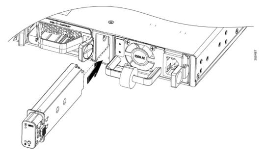
Figure 70: Installing an SSD Module on a Cisco Catalyst 9500 Series High Performance Switch
