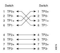
Figure 87: Two Twisted-Pair Straight-Through Cable Schematic
