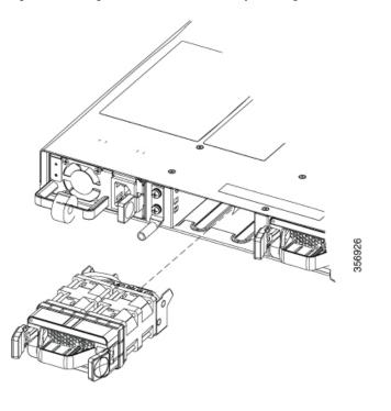
Figure 65: Installing the Fan Module on Cisco Catalyst 9500 High Performance C9500-32QC, C9500-48Y4C and C9500-24Y4C Switch Models
