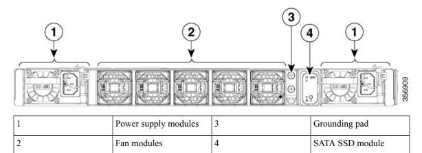
Figure 17: Rear Panel of a Cisco Catalyst 9500 High Performance Switch (C9500-32QC, C9500-48Y4C, and C9500-24Y4C)
