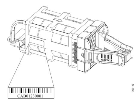
Figure 66: Fan Module Serial Number on Cisco Catalyst 9500 Series switches, High Performance Switch C9500-32C Switch and Cisco Catalyst 9500X Series C9500X-28C8D Switch Models
