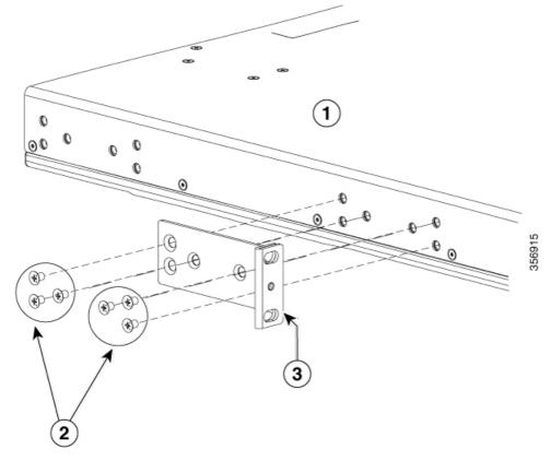
Figure 34: Middle Mounting position of Rack Mounting Brackets
