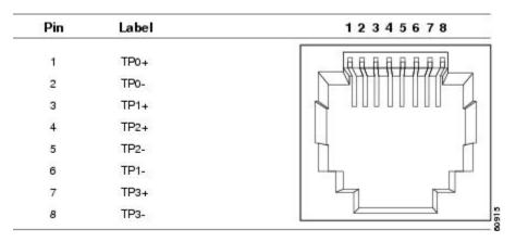
Figure 79: 10/100/1000 Port Pinouts
