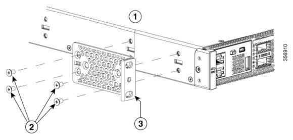
Figure 31: Middle Mounting position of Rack Mounting Brackets
