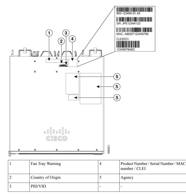
Figure 74: Serial Number Location Cisco Catalyst 9500X Series Switches
