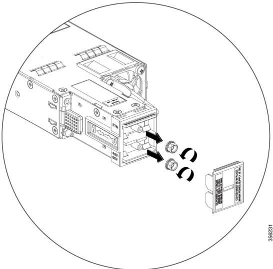
c. Secure the positive (+) DC power cable lug to the RTN terminal and the negative (-) DC power cable lug to the -48V terminal with the nuts.
