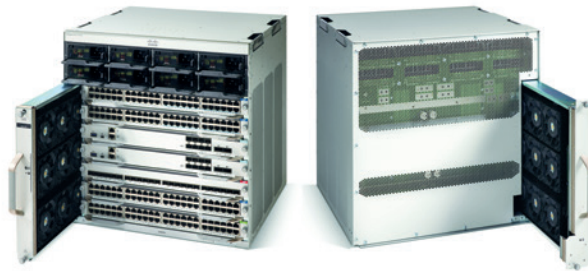
DIAGRAM Catalyst 9400 Series fan tray
