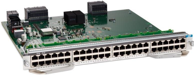
Figure 4. Cisco Catalyst 9400 Series 48-Port PoE+ 10/100/1000 (RJ-45) Line Card (C9400-LC-48P)
