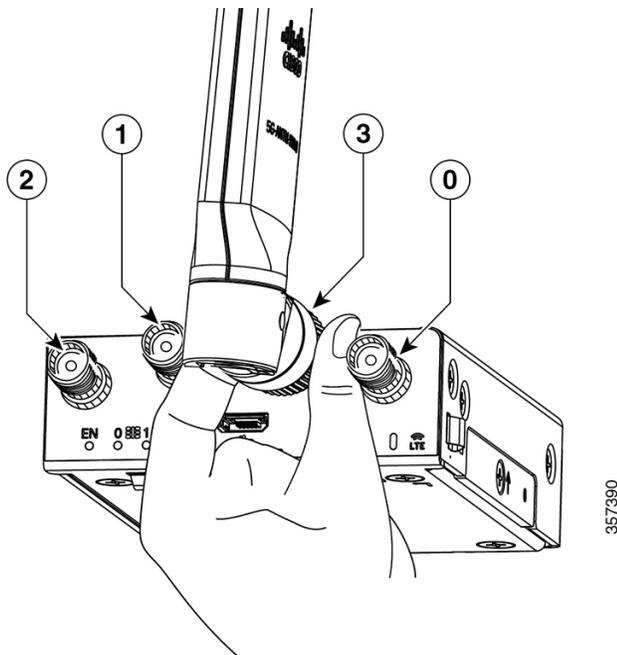
**Step 1** Use your thumb and index finger to insert and tighten antenna 1 and antenna 3 in the middle antenna attachment slots as indicated in the figure.
