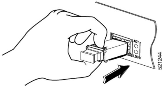
**Caution** Do not remove the optical port plugs from the SFP until you are ready to connect cabling.
