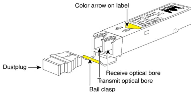
The CWDM SFPs come in eight wavelengths that range from 1470 nm to 1610 nm. Color markings on the devices identify the wavelength to which the Gigabit Ethernet channel is mapped. The table lists the SFPs with their wavelengths and color codes.
