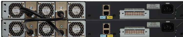
Figure 3. New StackWise-160 Modular Adapters and Stacking Cable
