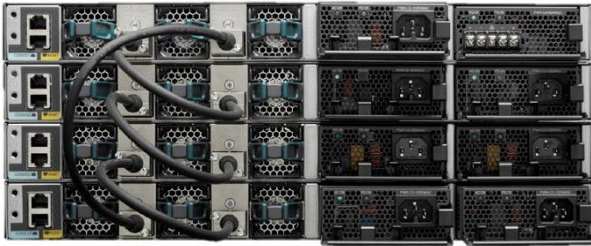
Figure 5. New StackWise-160 Modular Adapters and Stacking Cable
