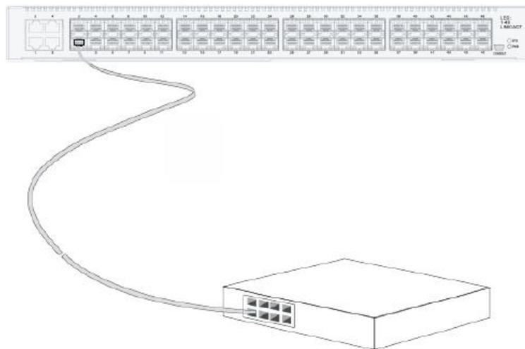
Figure 3-9 Connecting the gigabit SFP port and other Ethernet terminals
