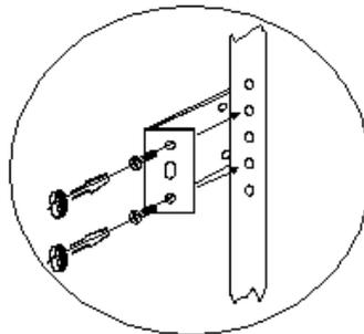
Figure 3-2 Installing the switch on the cabinet
