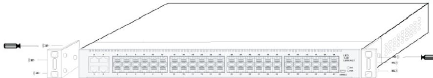
Figure 3-1 Fixing the machine box of the switch
