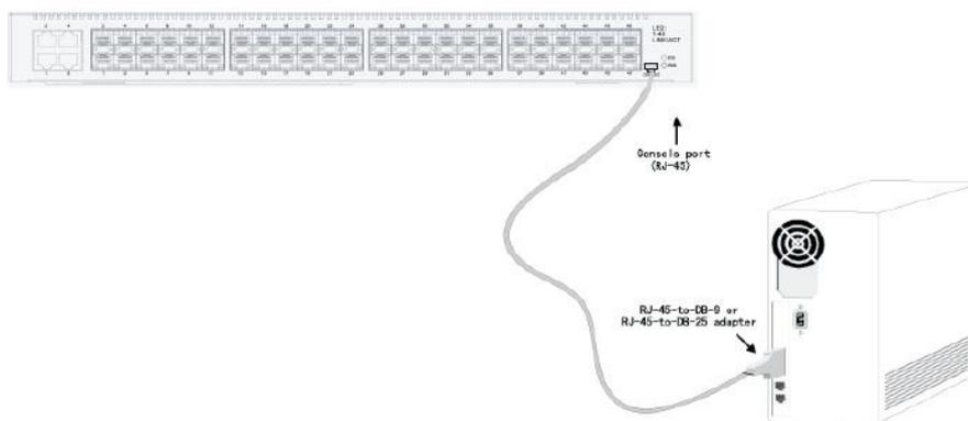
Figure 3-5 Connecting the console port of BDCOM S3756F and computer
