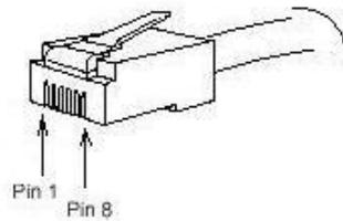
Figure 3-7 RJ-45 connector on the console port
