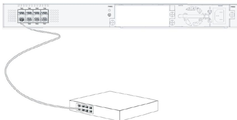
Figure 3-6 Connecting the 10G SFP+ port and other Ethernet terminals
