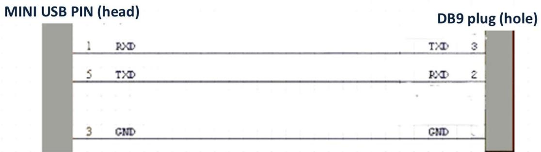
Figure 3-4 Cable connection at the console port
