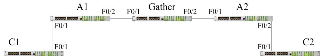
A1/A2/Gather belong to core network, C1/C2 are switches distributed in two places. Customer wants to combine two of its network to one , that is, the core network is a transparent transmission channel for the customer. If user wants to realize the
