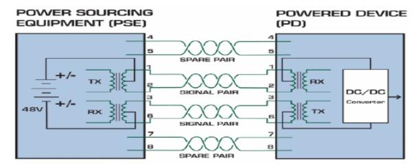
Generally speaking, standard PD has to support two power reception modes, while PSE only needs to support one of the two modes. All BDCOM products, as the PSE switches, only support the signal line power supply—alternative A.
