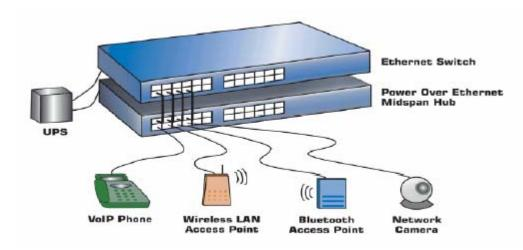
PI (Power Interface), the interface between PSE/PD and the network cable, is also defined in 802.3af. Up to now, there are two power supply modes defined: alternative A (signal lines, 1, 2, 3 and 6) and alternative B (idle lines 4, 5, 7 and 8).
