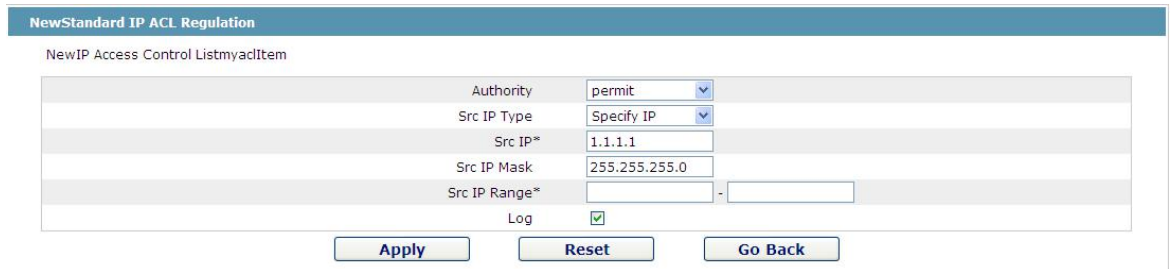
Figure 12: Setting the Rules of the standard IP access control list
