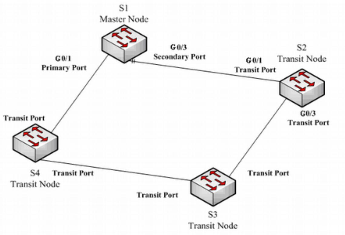
Figure 2.1 Fast Ethernet Ring Protection Configuration Example
