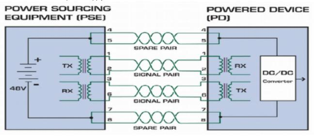
the cathode. The power supply is from PSE to PD.
