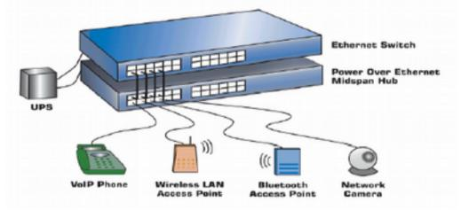
Meanwhile, 802.3af Standard also defines the PI (Power Interface: The interface between PSE/PD and network cable). At present, two power supply modes: Alternative A (Signal line No. 1, 2, 3, 6) and Alternative B (Free line 4, 5, 7, 8), have been defined, which are described as follows: 1) Supply the power through the idle pairs — Mode B (Alternative B)
