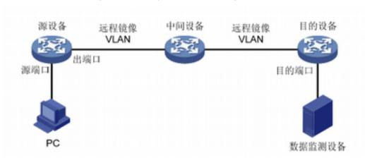
Configuring remote mirroring function on source device, and mirroring source port's message to the output port while adding configuring RSPAN TAG on the message. Vlan id in this tag is the remote mirroring VLAN. Middle device transfer mirroring message to the destination port by broadcasting. The destination device transfer
