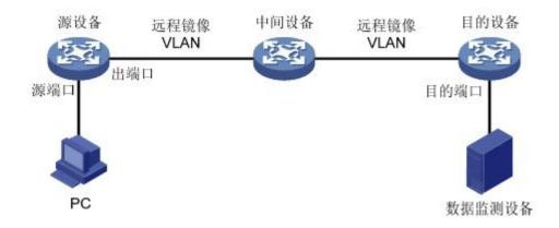
Configuring remote mirroring function on source device, and mirroring source port's message to the output port while adding configuring RSPAN TAG on the message. Vlan id in this tag is the remote mirroring VLAN. Middle device transfer mirroring message to the destination port by broadcasting. The destination device transfer message from
