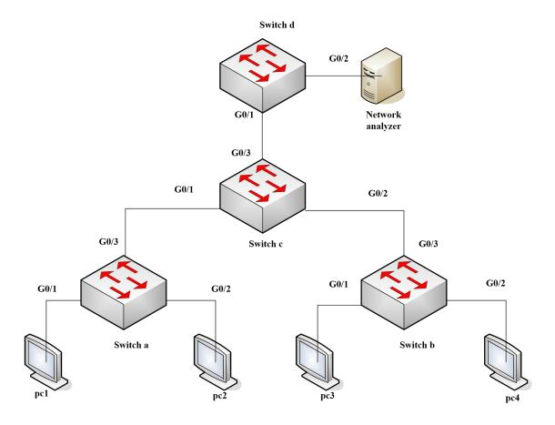
You need to monitor the traffic of interface g0/1 on switch a and interface g0/1 on switch b by the network analysis meter.
