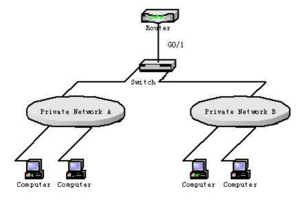
(1) Enable MACFF in VLAN1, which connects private network A. The default gateway allocated by DHCP server is 192.168.2.1.
