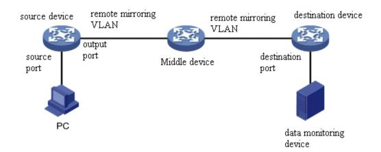
Configuring remote mirroring function on source device, and mirroring source port's message to the output port while adding configuring RSPAN TAG on the message. Vlan id in this tag is the remote mirroring VLAN. Middle device transfer mirroring message to the destination port by broadcasting. The destination device
