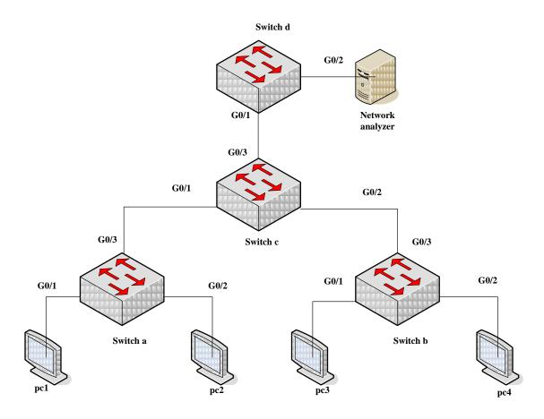
Users need to monitor the flow of the g0/1 port in switch a and the g0/1 port in switch b at the network analyzer, which can be realize through remote mirroring. The configuration is as follows:
