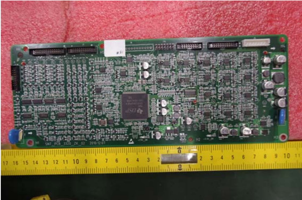
Fig.19 –Board PCB_3320_CT2, traces side view
