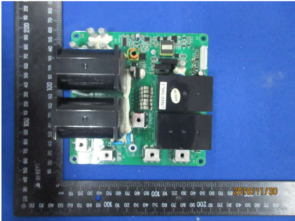
Figure 25: PCB component view
