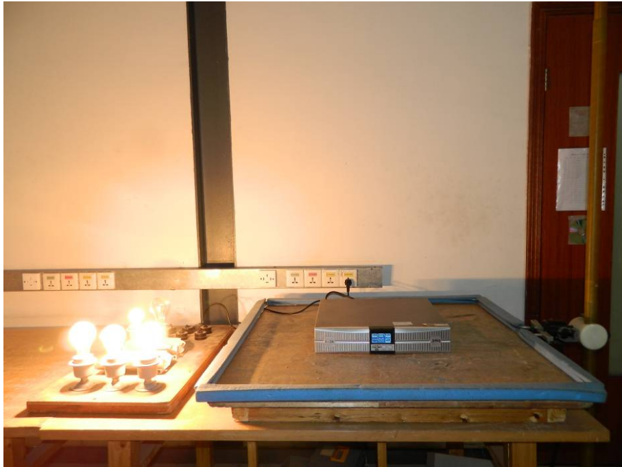
17.9.Photo of Magnetic Field Immunity Test
