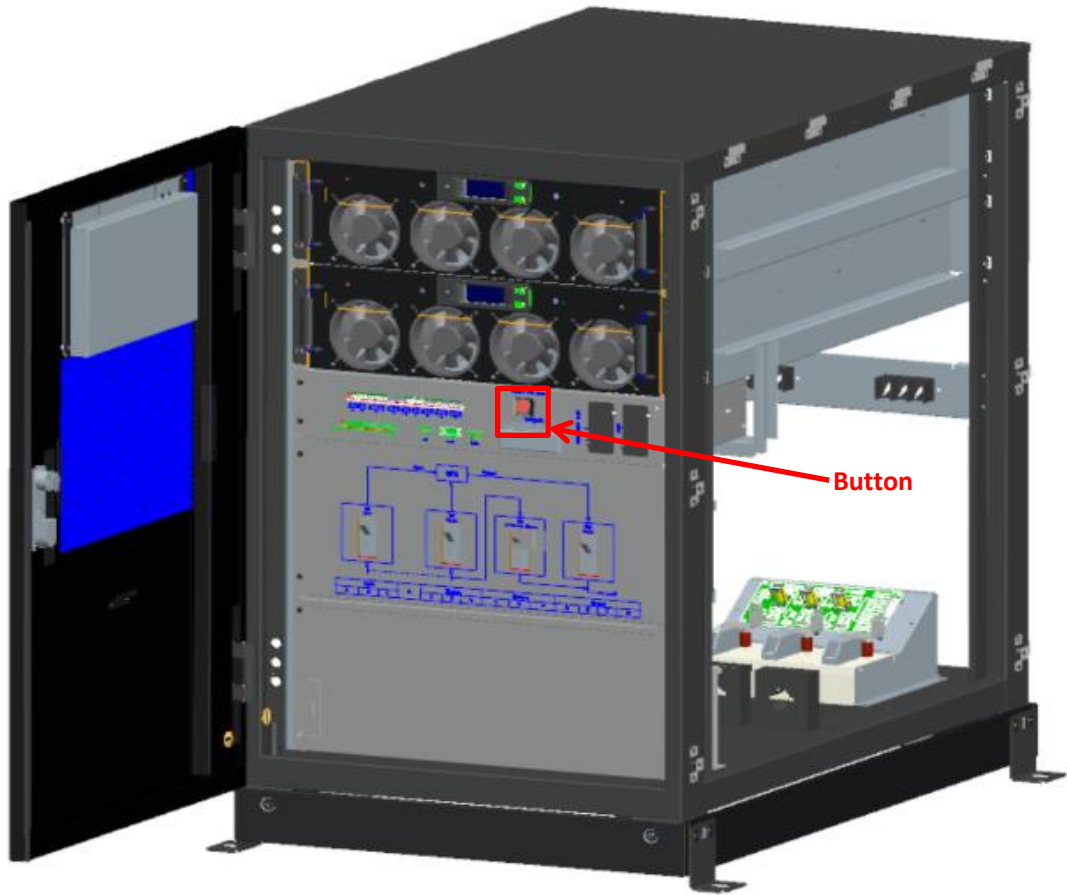
Figure 3 button installation place
