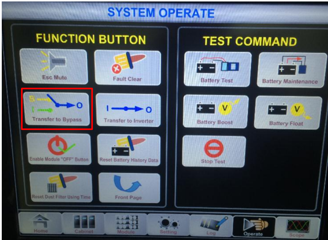
Figure 11 Manual bypass function
