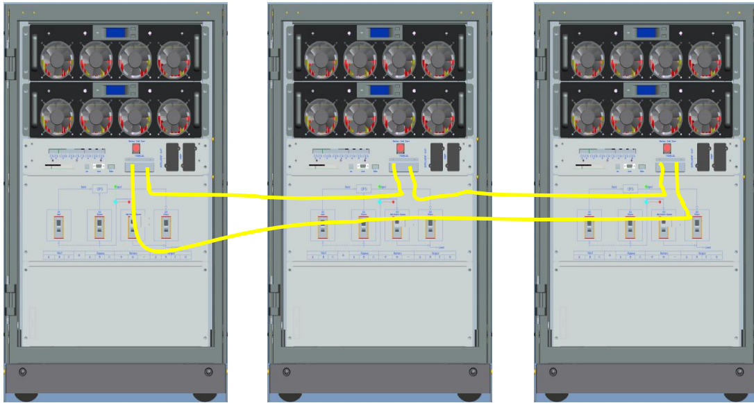
Figure 6 Parallel signal cables connection
