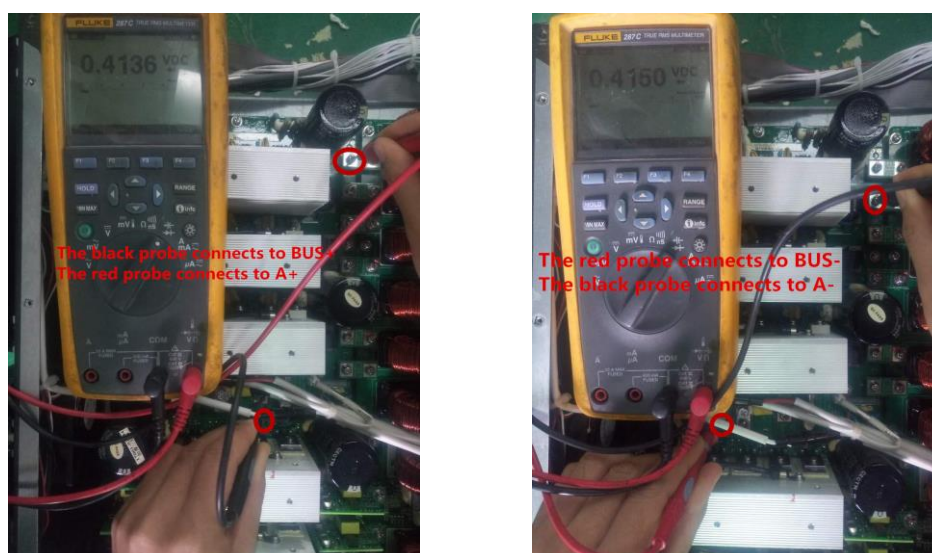
Figure 4.3 Rectifier IGBT pin test
