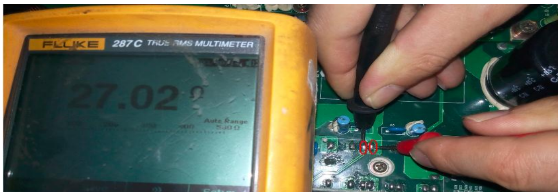
Figure 6-1 Normal resistance of the rectifier SCR
