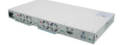
This model of power supply is systemic one which features wide input voltage range, output voltage 54.5V, max output current 5A for single rectified module, and floating charge for battery. System has two rectified modules which are integrated, and then output. Output voltage refers to voltage after integration. There is a monitoring module that communicates with supervisory control computer by RS232 to monitor power supply and battery.
