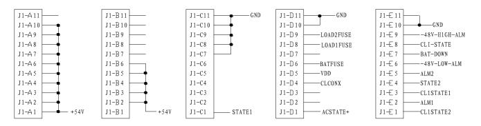
A1-A10: +54V is the positive terminal of the 54V DC input.
