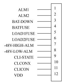
1. ALM1 is the collector input of output warning OPT of rectification module 1, high resistance for warning status and low electric level for normal operation
