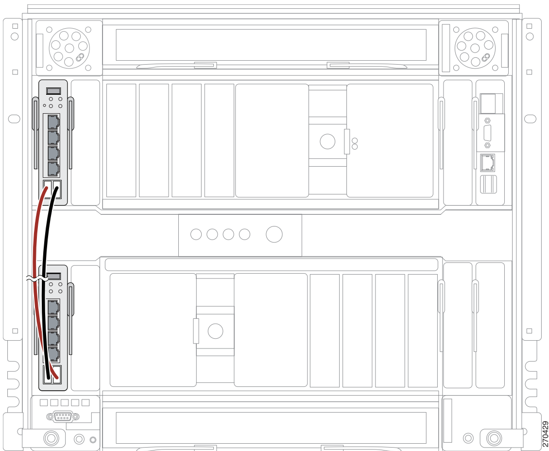
Figure 12 Switch Stack Cabling Example
