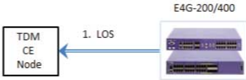
Figure 19: LOS Alarm Generation
