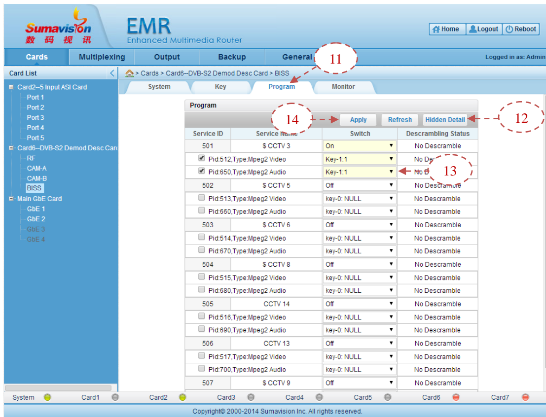
Fig. 5-106 DVB-S2 Demod Desc Card BISS Descrambling Program Setting
