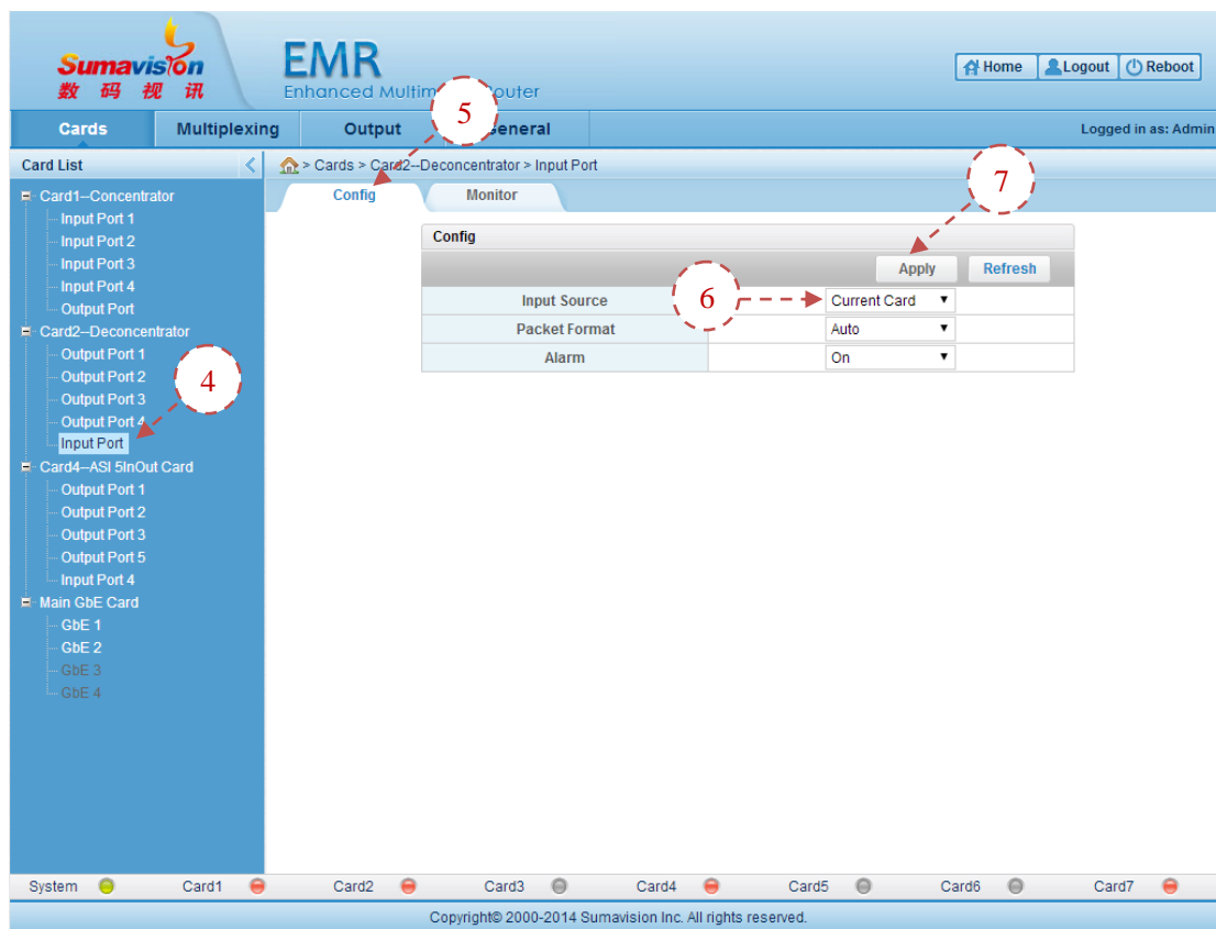
Fig. 5-43 ASI 5InOut Card Deconcentrator Input Settings
