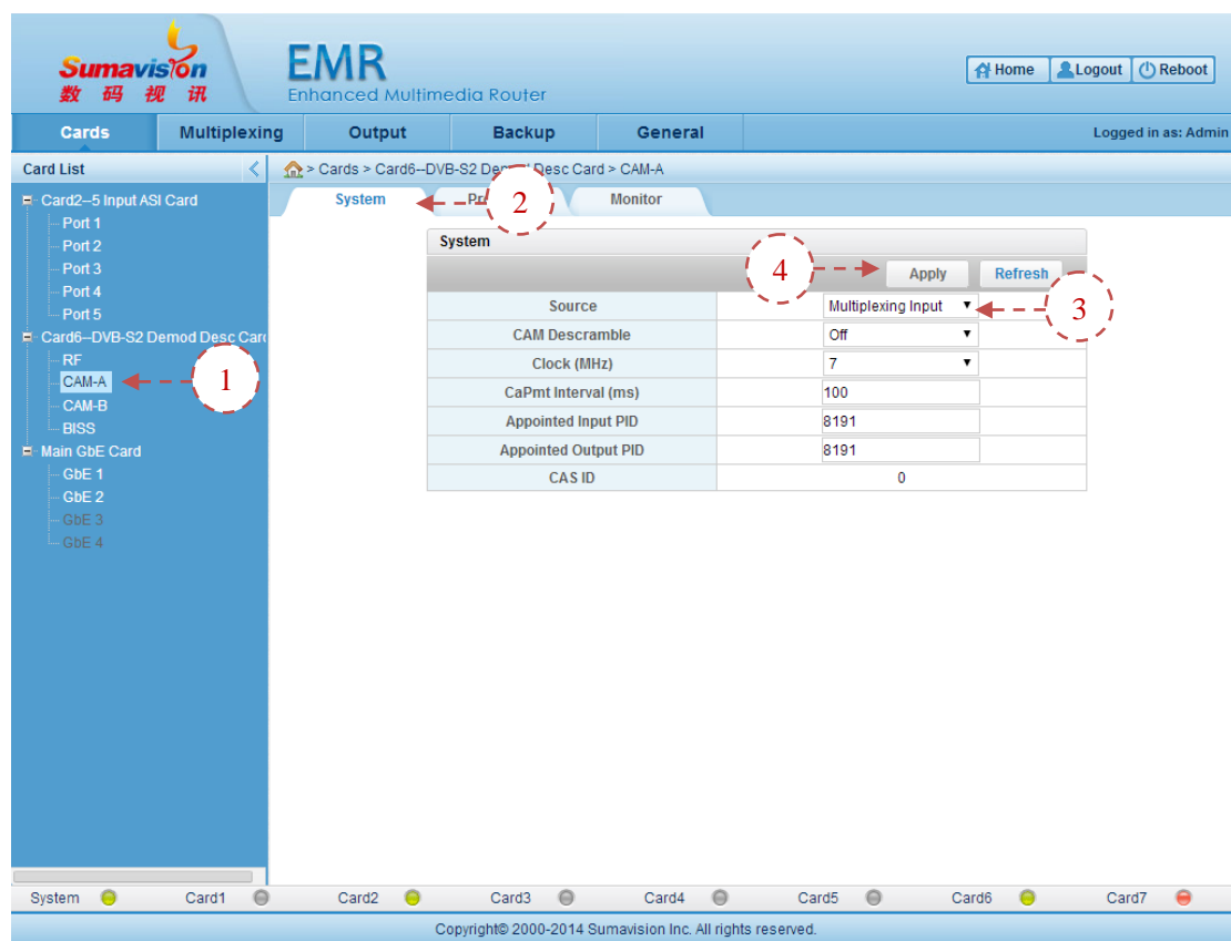
Fig. 5-101 DVB-S2 Demod Desc Card CAM Descrambling System Parameter Setting
