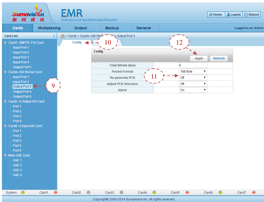
Fig. 5-39 ASI 5InOut Card Output Settings
