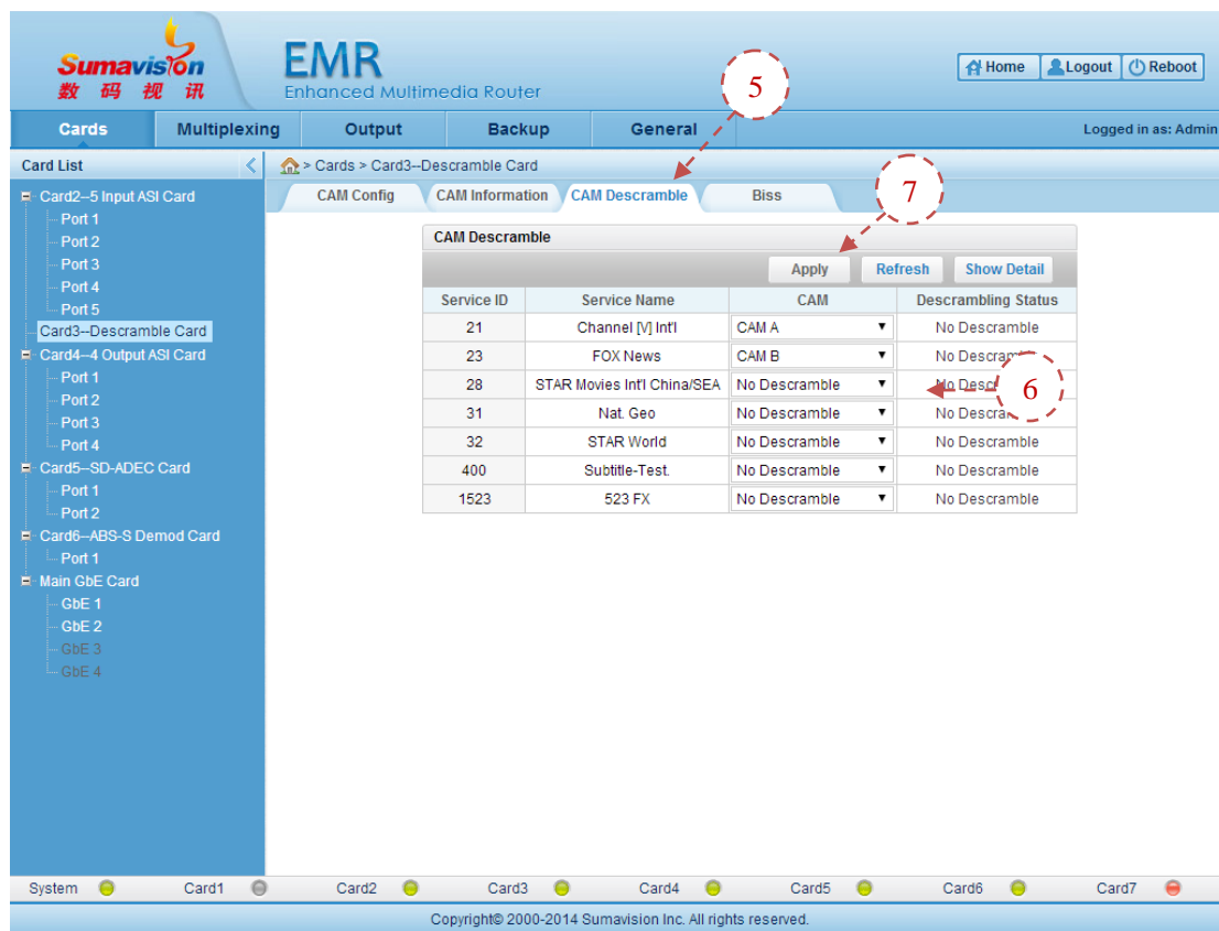
Fig. 5-79 Descramble Card CAM Descrambling
