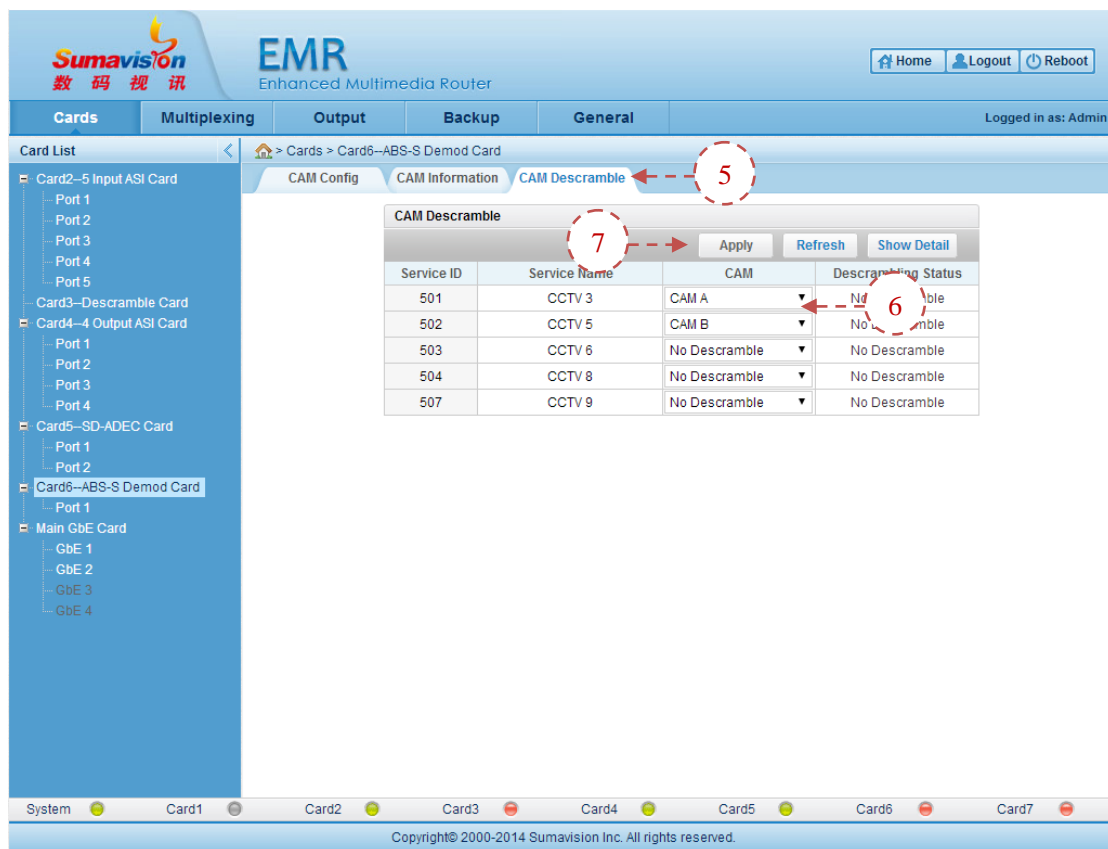
Fig. 5-91 ABS-S Demod Card CAM Descramble
