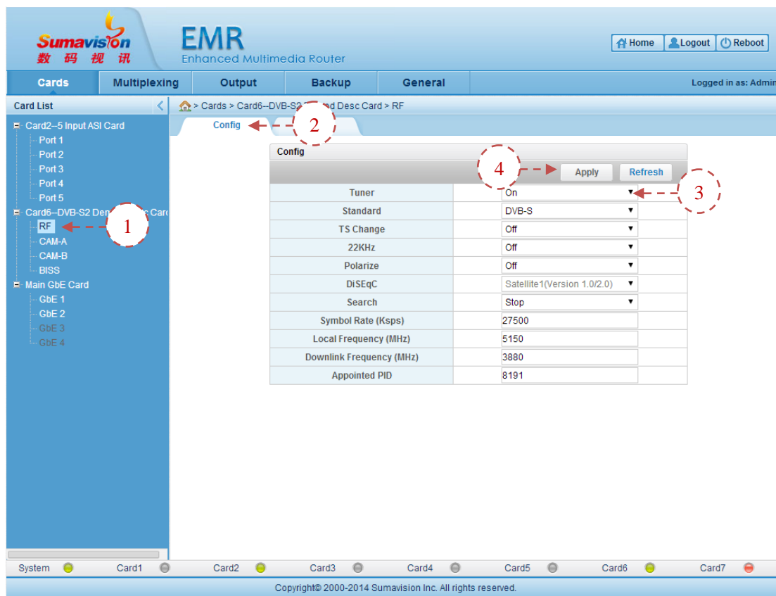
Fig. 5-99 DVB-S2 Demod Desc Card Receiving Parameter Config
