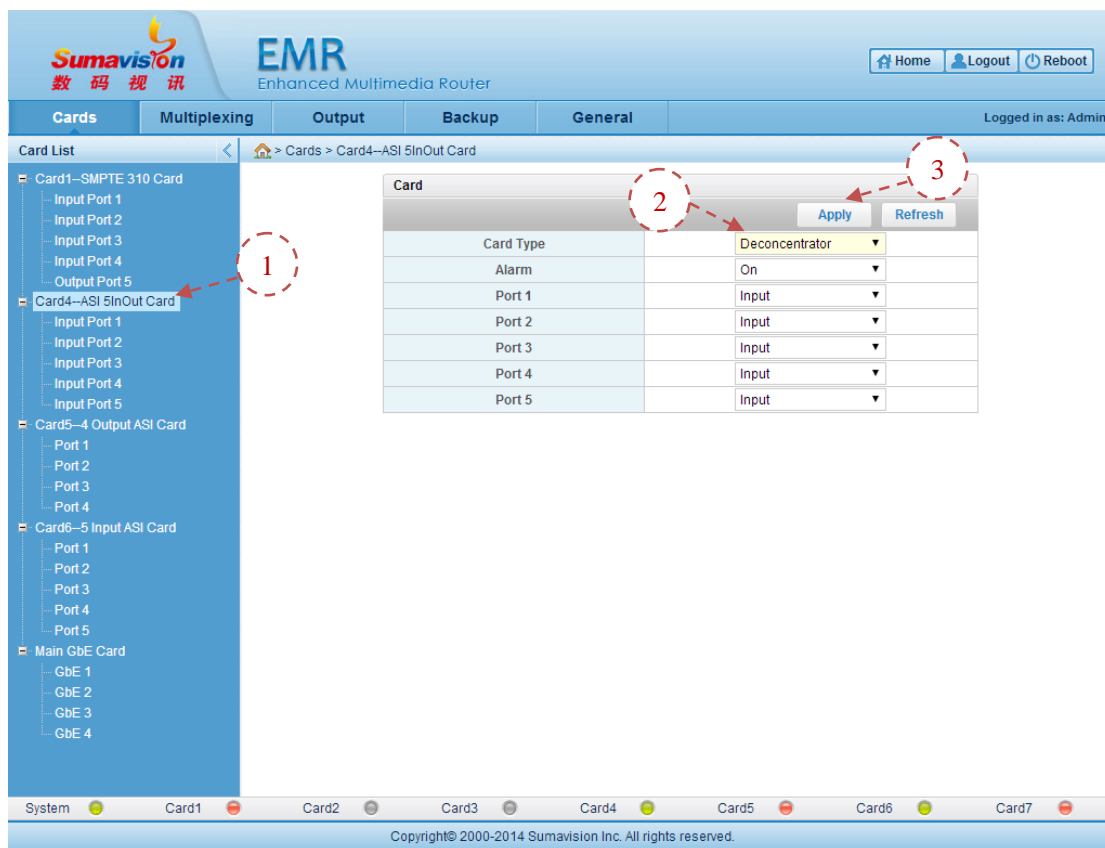
Fig. 5-42 ASI 5InOut Card Deconcentrator
