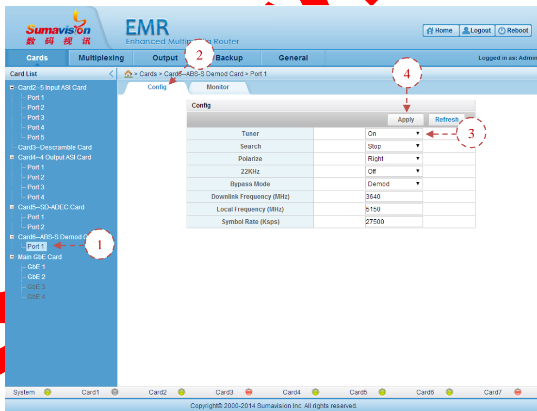
Fig. 5-89 ABS-S Demod Card Receiving Parameter
