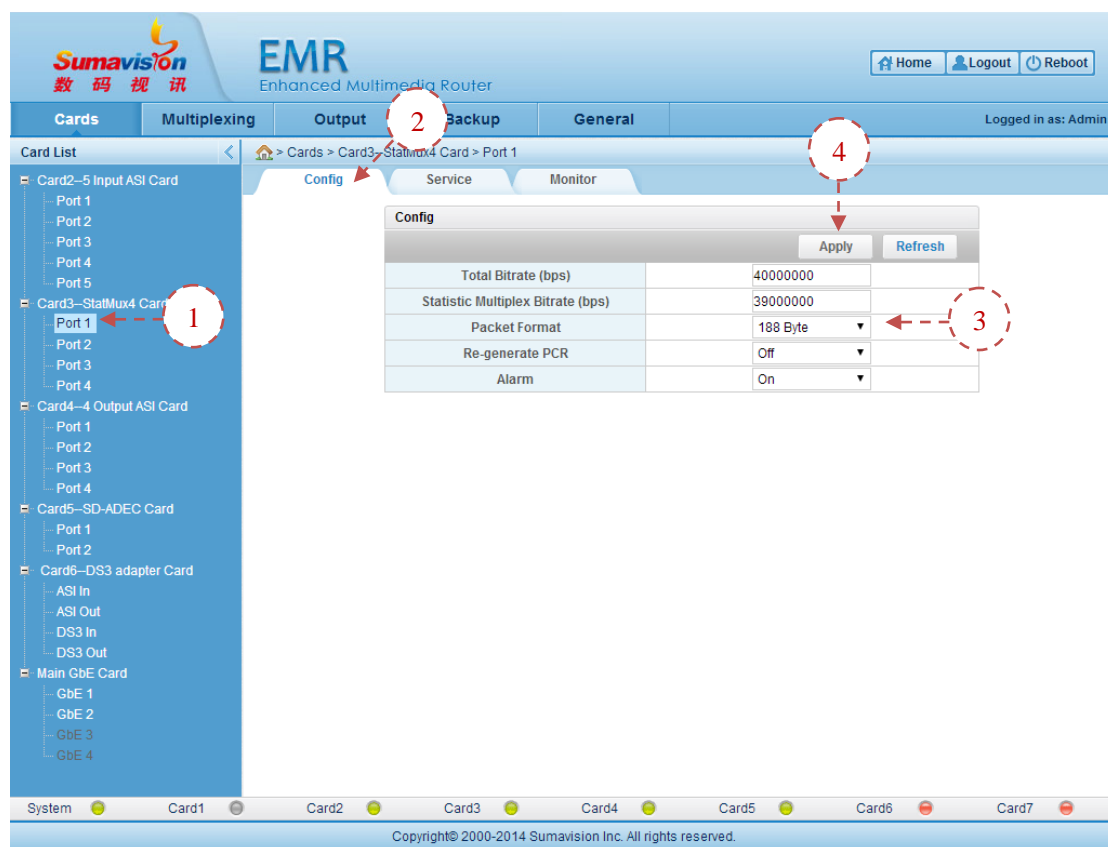
Fig. 5-118 StatMux4 Card Port Config
