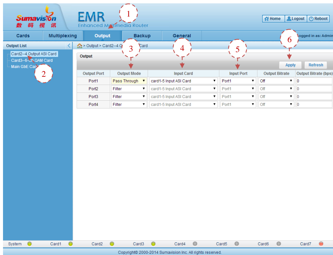
Fig. 6-39 Output Setting Interface for Web Network management
