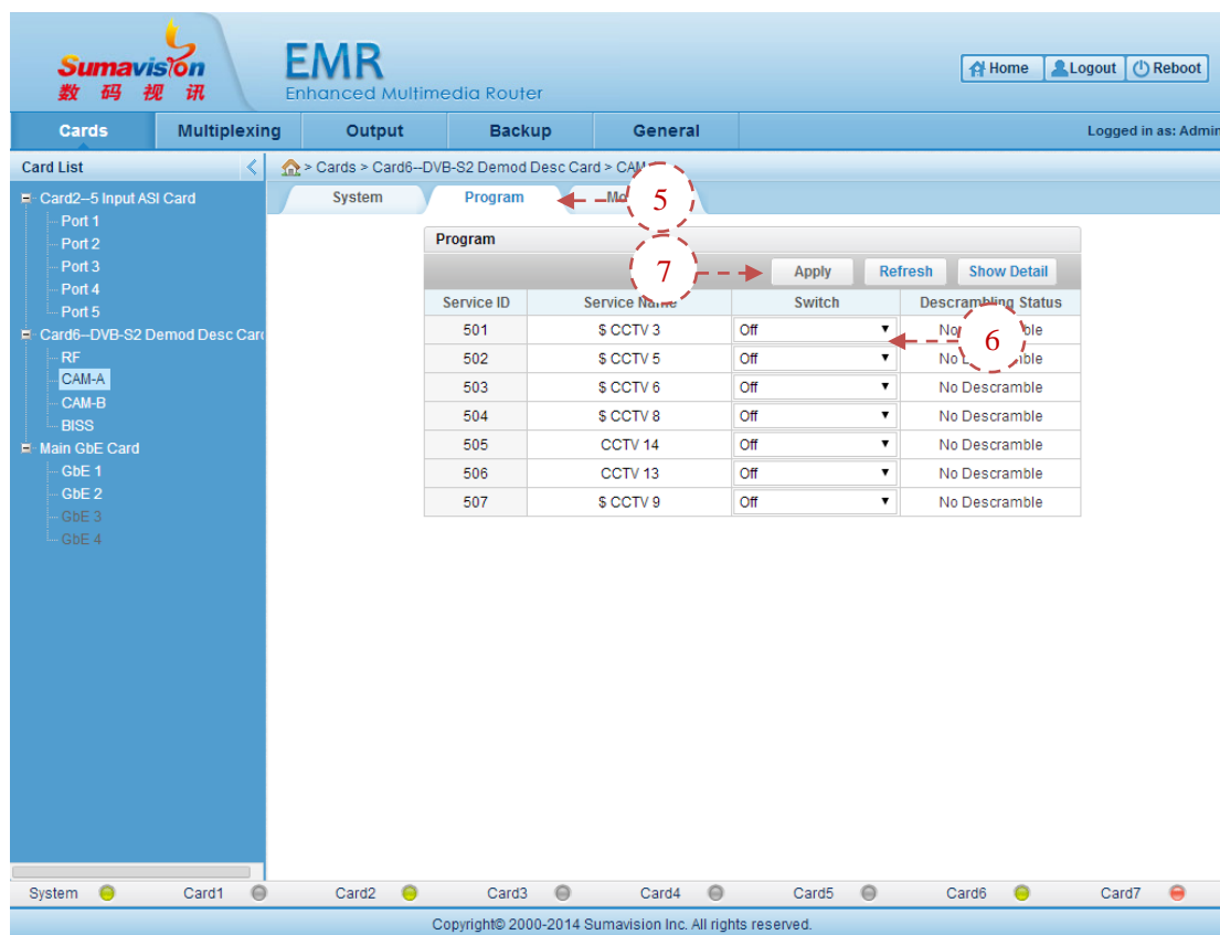
Fig. 5-102 DVB-S2 Demod Desc Card CAM Descrambling Program Setting
