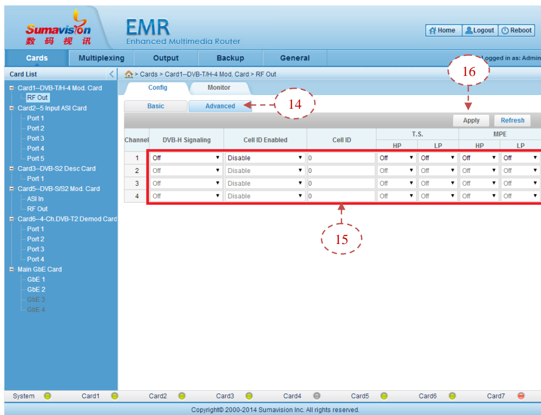
Fig. 5-61 DVB-T/H-4 Mod. Card RF Out Config Advanced Parameter Setting
