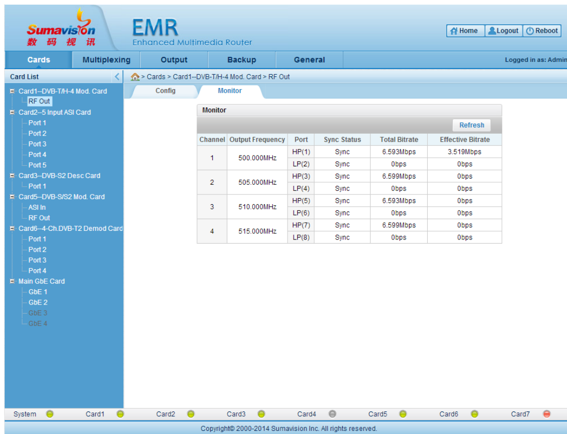
Fig. 5-62 DVB-T/H-4 Mod. Card RF Out Monitor
