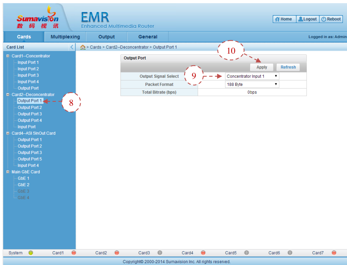
Fig. 5-44 ASI 5InOut Card Deconcentrator Output Settings
