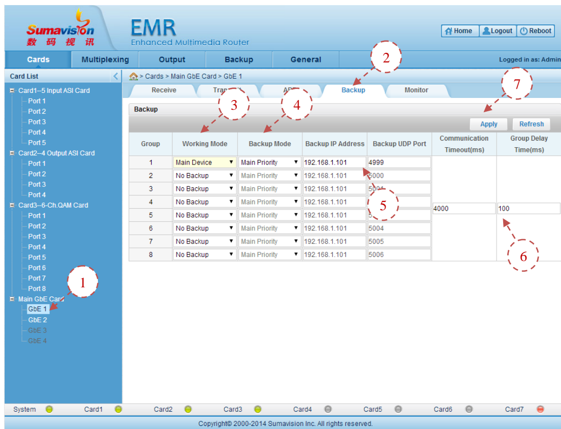
Fig. 5-30 Main GbE Card Output port Backup
