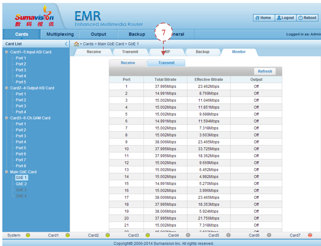
Fig. 5-25 Main GbE Card Transmit Monitor
