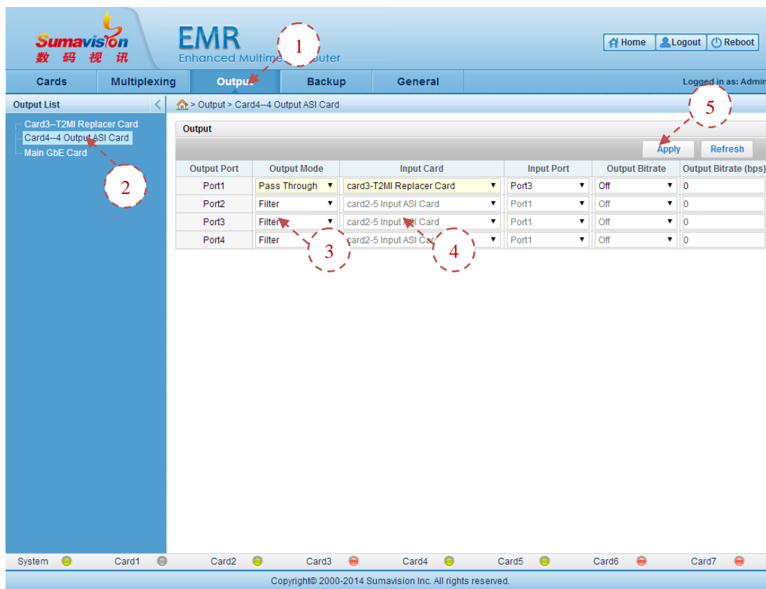
Fig. 5-147 T2MI Replacer Card Output via Other Cards
