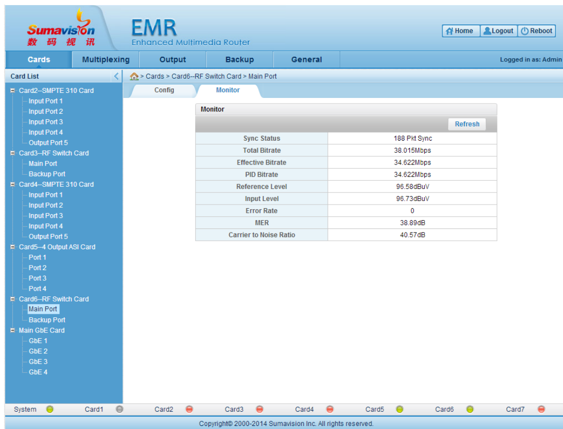
Fig. 5-138 RF Switch Card Port Monitor
