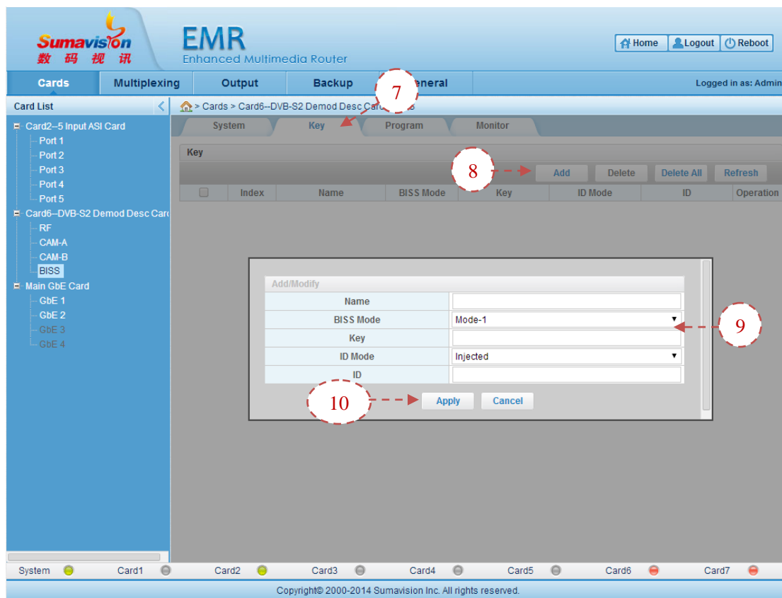
Fig. 5-105 DVB-S2 Demod Desc Card BISS Descrambling Key Setting
