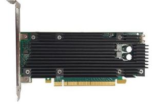
(LCC) based Xeon-D servers. The commercial solution shall be implemented on the Low profile half-length PCle x16 Gen-3 PCle add-in card.
