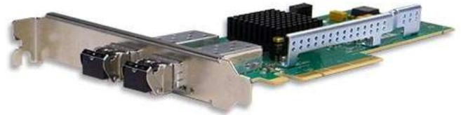
The Silicom 25 Gigabit Ethernet PCI Express server adapters are based on Broadcom BCM57304 Ethernet controller with fully integrated Gigabit Ethernet Media Access Control (MAC) and SFI Interface. In addition to managing MAC and PHY Ethernet layer functions, the controller manages PCI Express packet traffic across its transaction, link, and physical/logical layers.
