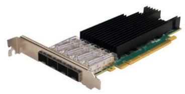
The Silicom 25 Gigabit Ethernet PCI Express server adapters are based on Intel XXV710 Ethernet
