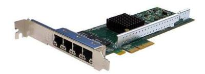
Silicom's Quad Port Copper Gigabit Ethernet PCI Express
